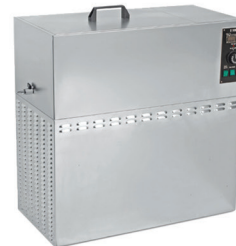
CURING BATH WITH COOLING UNIT
